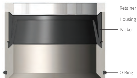
Standard Pressure Sealing Assembly
