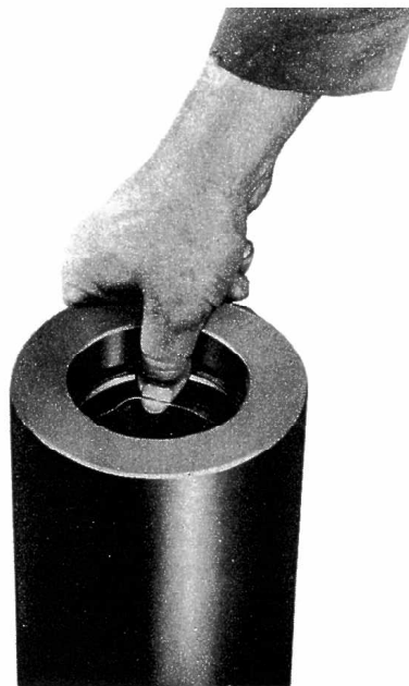
Figure 16 Insert one edge into the groove. Then insert the opposite edge and press down until the entire ring is in place.
