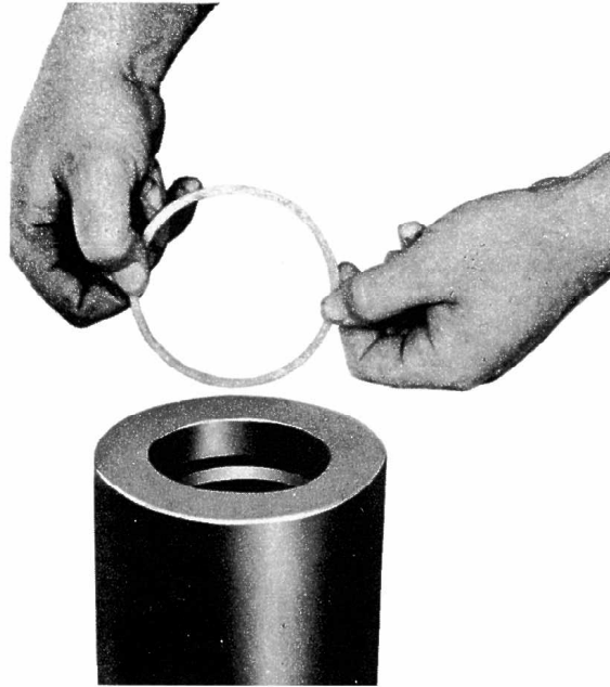
Figure 14 Ring is shown before being bent. It will look like this after it is properly installed in the groove.
