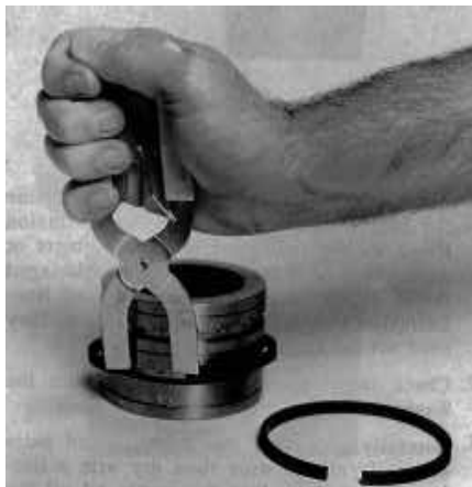
Figure 7 Piston Ring Removal
