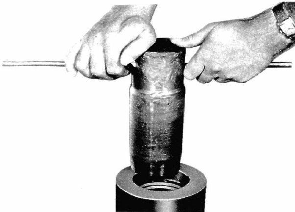
Figure 23 Insert the setting tool as shown. Use any convenient rod or bar to hold the tool.
