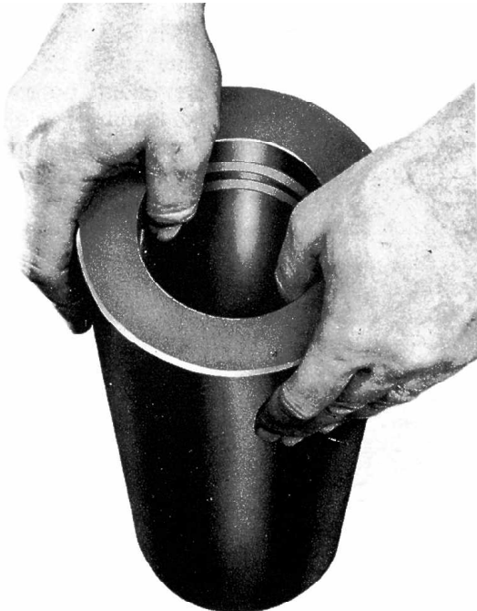
Figure 13 Using thumbs, press ring into groove until ends match up and ring is firmly seated in the groove.
