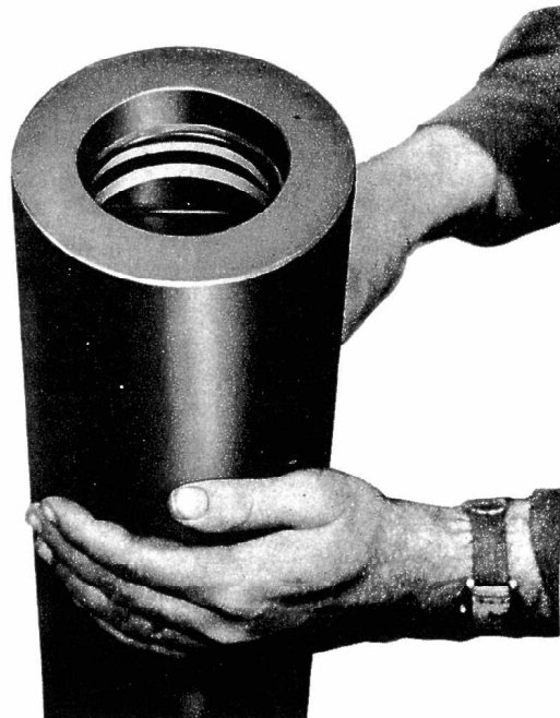
Figure 20 Insert O-Rings between Seal Protection Rings in each groove.
