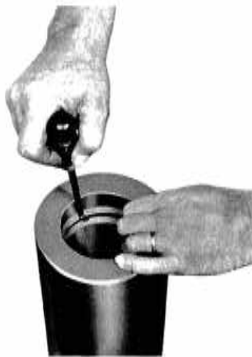
Figure 8 Seal Assembly Removal
