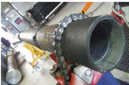
A new string-dynamics logging tool can be integrated most workstring setups, recording tension, compression, torque, temperature, and internal and external pressure. (Image courtesy of NOV)
