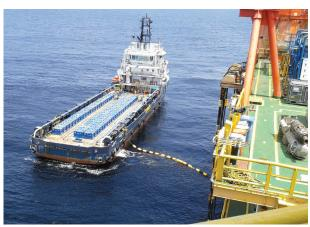
The NOV FluidControl cuttings transfer and containment solution enabled safe, effective and efficient management of our clients drilling waste as they transitioned to a Zero-Discharge drilling application offshore.
