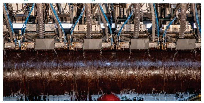
Oilfield tubulars with advanced performance properties demand a more sophisticated inspection method beyond traditional ultrasonic techniques. Utilizing leading-edge Phased-Array technology Tuboscope identifies pipe flaws at multiple orientations along with over 100% UT wall coverage for higher accuracy and reproducibility.
