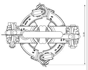
The D-SJX is the heavy duty version of the SJX, capable of handling doubles and triples up to 12 STon / 10.9 Tonne.
