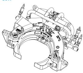
The SJH horizontal pick up elevator is designed to pick up tubulars lying flat on a surface without having to lift the tubulars prior to closing the elevator. The elevator is capable of lift ing drill pipe, recessed/zip lift drill collars and casing. It will handle single joints of pipe straight from cantilever to off-line stand building systems.
