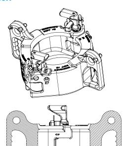
The SJX single joint elevator is designed for running single joints of tubing and casing from V-door to well center. It is double hinged for use with the CRT Casing Running Tool, or any other stabberless operation. Ergonomically designed handles with cast on stop pins prevent the lifting sling shackles from pinching hands. Suitable for loads up to 5 sTon / 4.5 Tonne.
