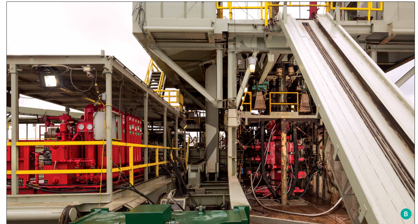
B. Same BOP stack pictured on left-hand page on rig
