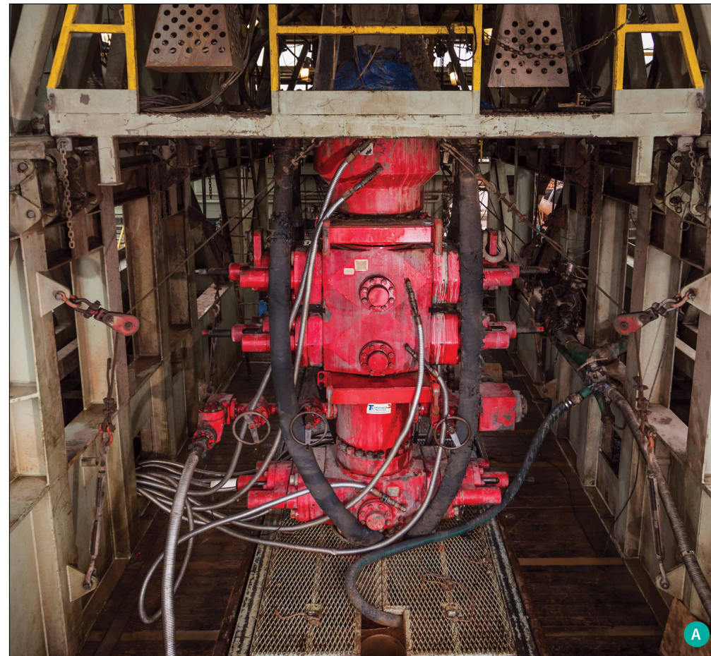
A. BOP stack: 6012 Single Ram (bottom), 6012 Double Ram (middle), Spherical (top)
