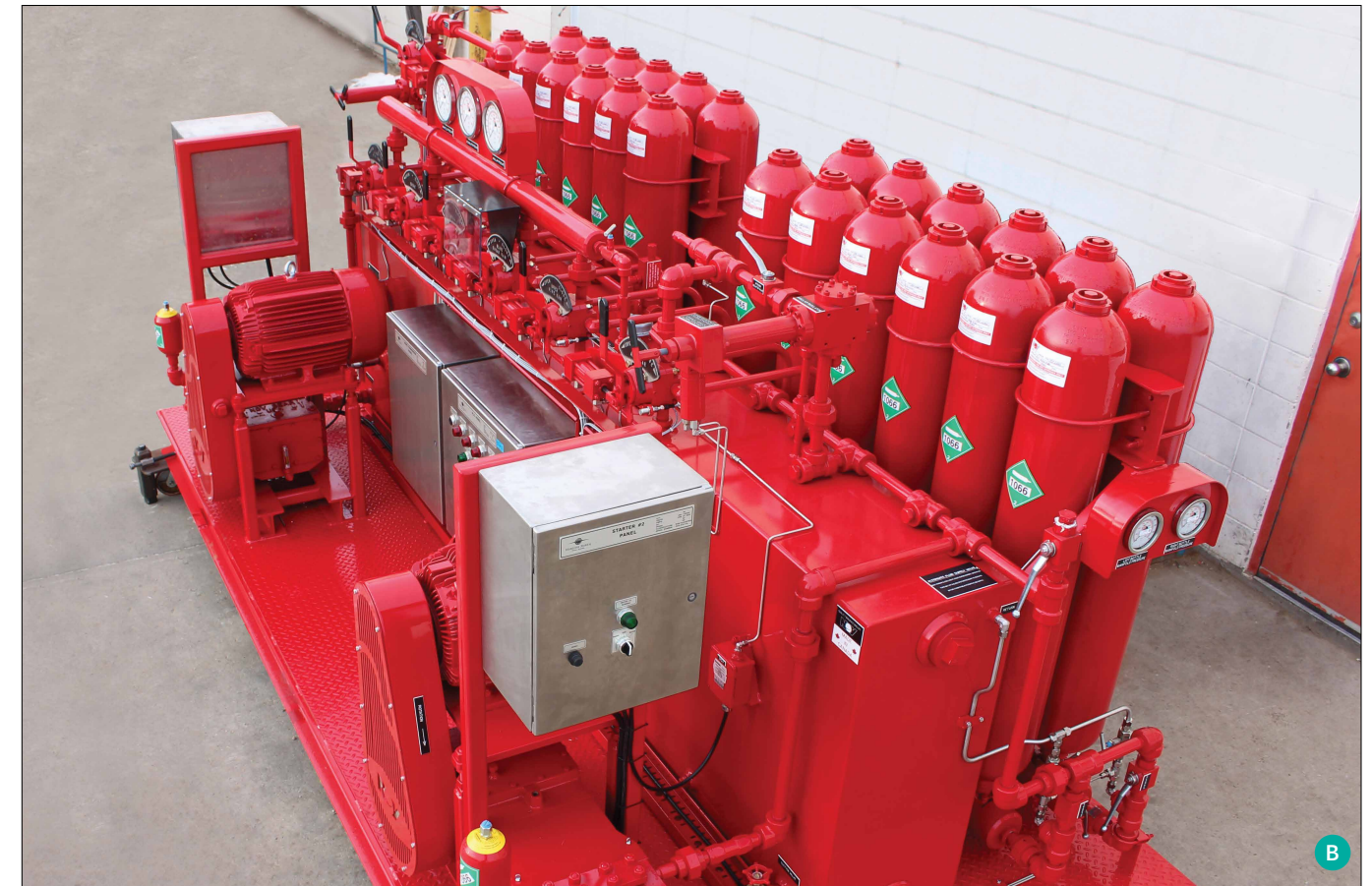
B. BOP Control System Unit
