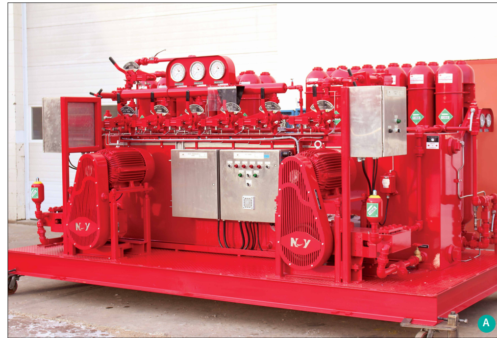
A. BOP Control System Unit
