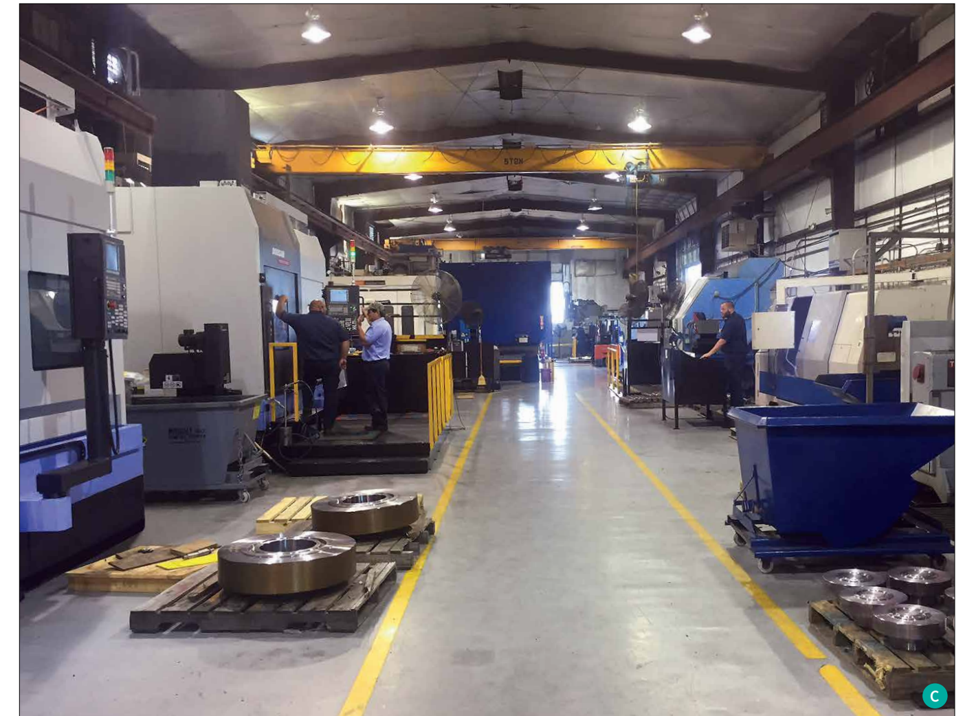
C. Facility Floor with CNC Vertical Mills on left-hand side and CNC Lathes on the right-hand side
