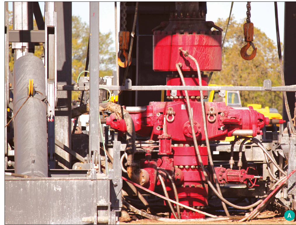
A. BOP stack: LXT Single Ram BOP (bottom) and Spherical BOP (top)
