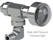
Packing rings in the lower rotating housing of a washpipe cartridge fail sequentially. Once the third packing ring begins to leak and the fourth packing ring energizes, the light will begin to strobe; this indicates that the washpipe packing needs to be replaced at the soonest opportunity. The early warning provided by the Blak-JAK Pressure Indicator light can consistently prevent mud leakage and unnecessary downtime. For more information contact your NOV MISSION representative.
