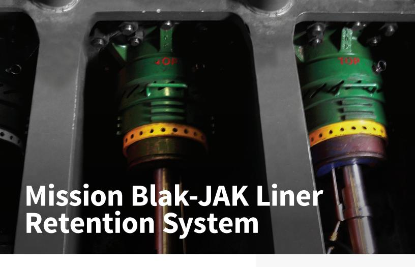
The Mission™ Blak-JAK™ liner retention system consists of two cellular components for ease of use: the Lok-CEL™, which mechanically retains the liner while the pump is in operation, and the Hydra-CEL™, the removable hydraulic assist that places the Lok-CEL in tension while simultaneously placing the liner in compression. Our designs improve fluid end maintenance procedures, reduce risk exposure, and speed up liner change-out times.
