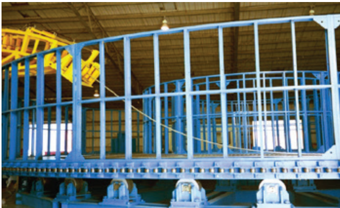
Tube umbilical loading into basket carousel using natural catenary from loading arm.
