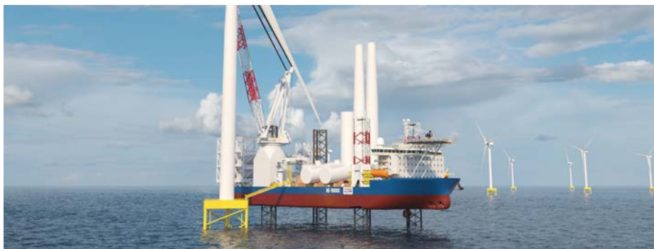
Stable installation of next generation WTG's. High height reach for max. 161 m
