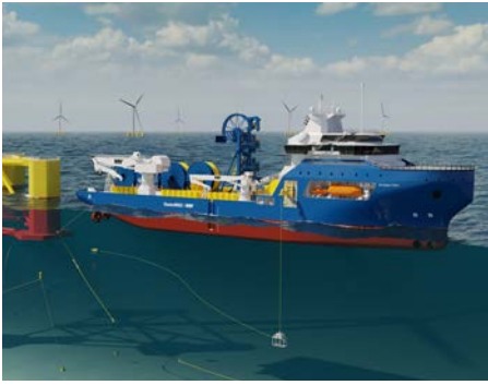
Enhydra FWIV - mooring operations
