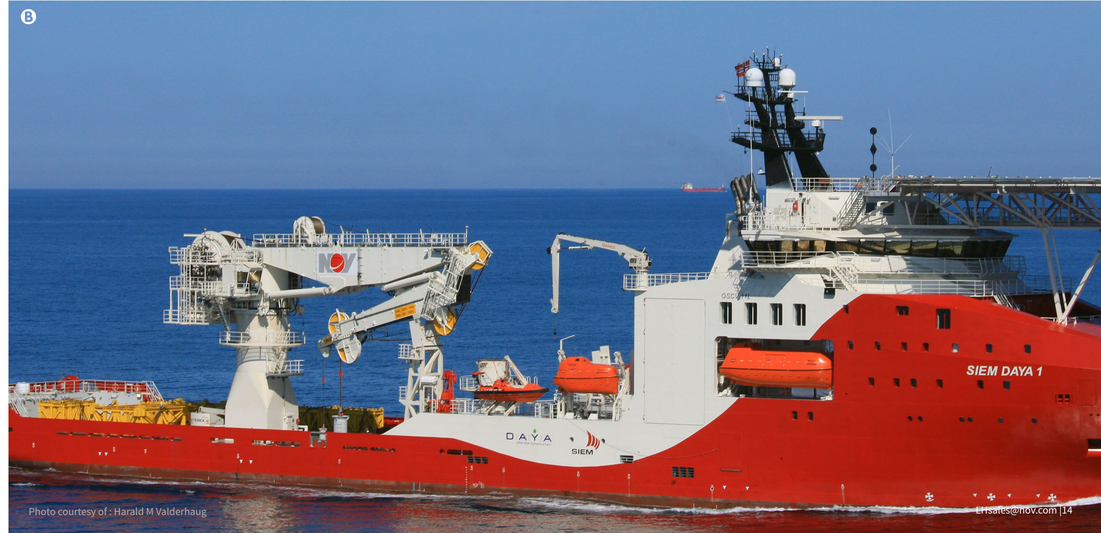
A - MSB Crane on Normand Maximus B - 250 t OCKS crane on Siem Daya 1 C - 400 t OCKS crane on Normand Clipper
