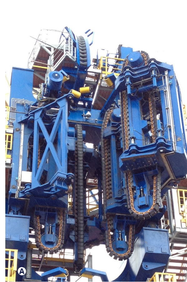
A - 90 te 4 track VLS tensioner B - 15 te side loading horizontal 2 track tensioner C - 70 te (2 x 35) tensioners tandem mounted for a dual lay capability
