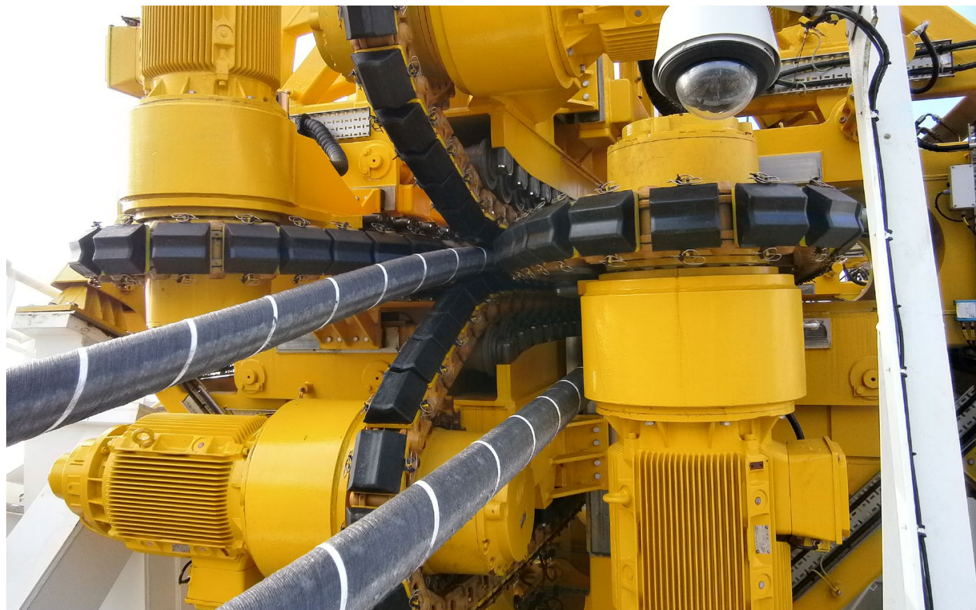
35te - 4 track multi-orientation tensioner with dual lay capacity
