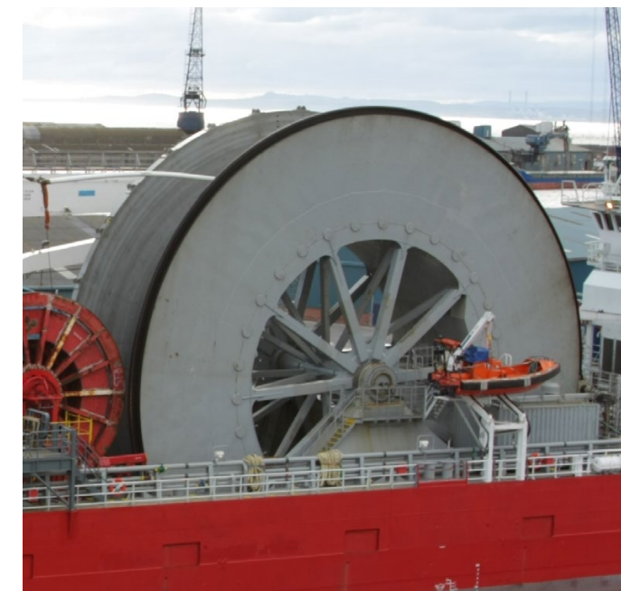
Integrated horizontal axis reel
