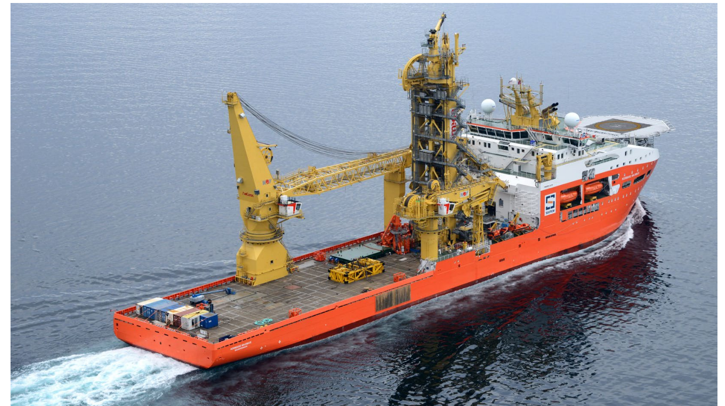
900 t MSB-S crane on Normand Maximus | Photo courtesy of: Harald M. Valderhaug
