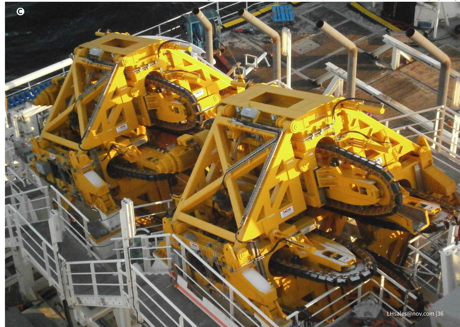
A - 90 te 4 track VLS tensioner B - 15 te side loading horizontal 2 track tensioner C - 70 te (2 x 35) tensioners tandem mounted for a dual lay capability
