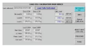
Load cell three-point calibration HMI
