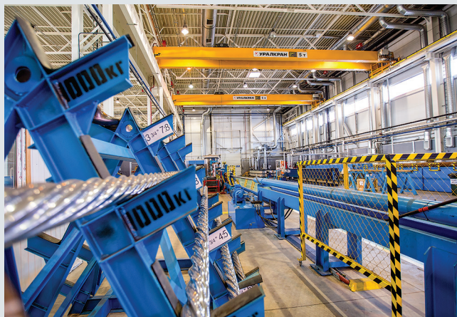
Fig. 2. NOV's 137,795-ft 2 manufacturing facility was built to address the unique needs of the Russian market. In addition to land rigs, the facility also manufactures drill bits, downhole motors and underreamers, fishing tools, drilling jars and completion tools. Photo: NOV.
