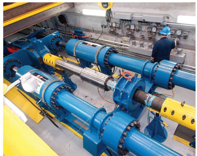
Fig. 3. A full-scale simulator performed combined load testing, which ensured adherence to API standards.
