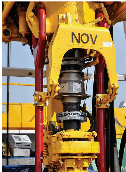
Fig. 1. A direct drillstring measurement sensor was integrated into a standard top drive internal blowout preventer.
