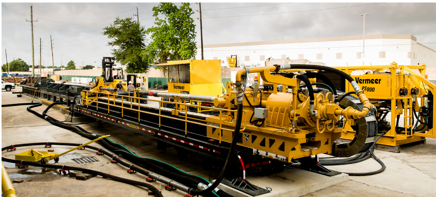
Figure 2. The Horizontal Milling Machine (HMM) from NOV aids in the simulation of well environments while quantitatively measuring tool performance.
