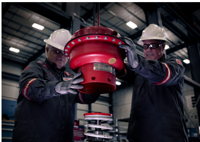
Figure 3. Two NOV service technicians inspect a fail-safe pneumatic actuator.
