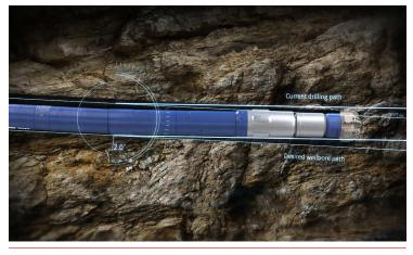
Figure 2. Vector Series 50 SelectShift downhole adjustable motor.
