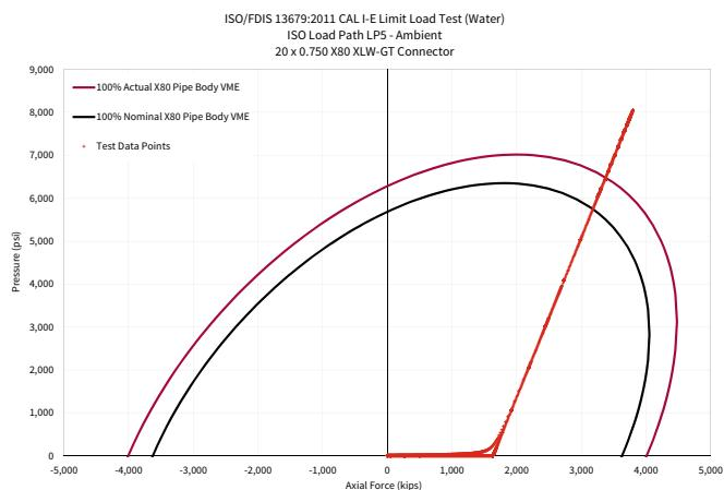
Successfully qualified to 95% of X80 actual pipe body internal pressure ratings to ISO/FDIS 13679:2011 CAL I-E (with gas)
