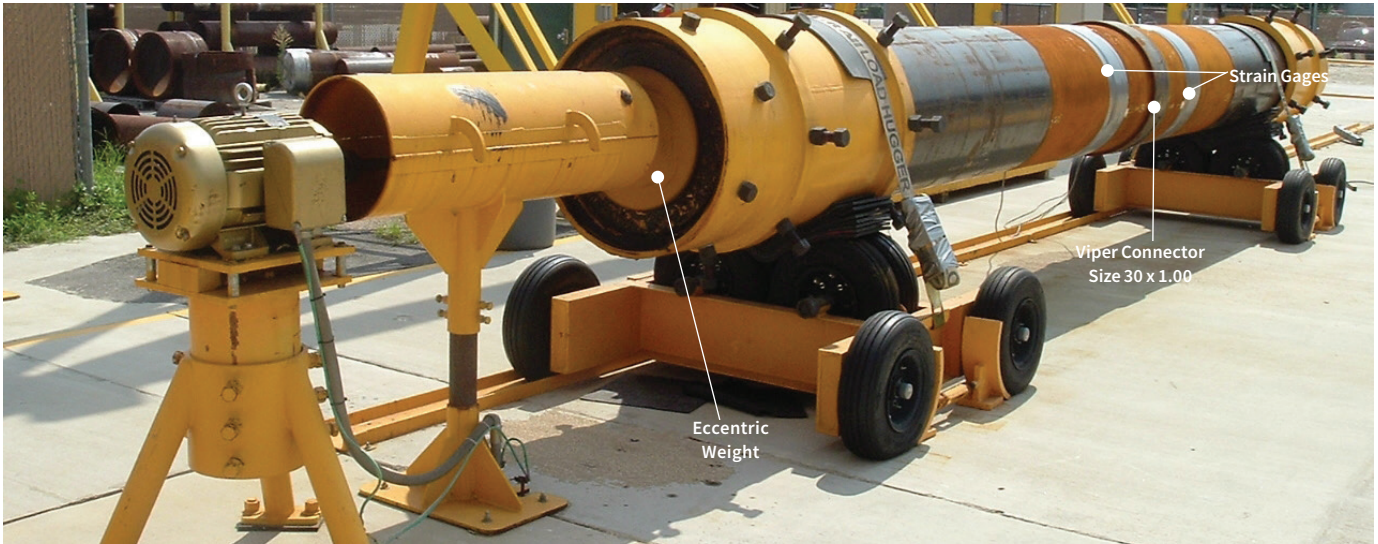
Figure 1: Harmonic Fatigue Testing Assembly
