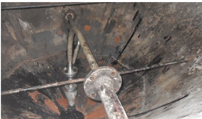
Figure: ToreScrub sand cleaning unit located next to the heater treaters (top). ToreOVD fluidization device in treater (bottom).
