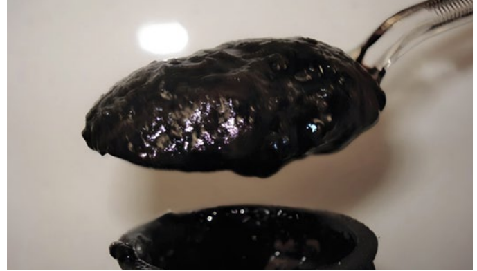
Figure: Oily sludge removed from heater-treaters.
