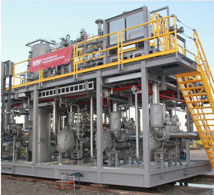
Operator/Project: Hess, Stampede Tension Leg Platform Solutions Provided: Fuel Gas Conditioning Package Year Delivered: 2015
