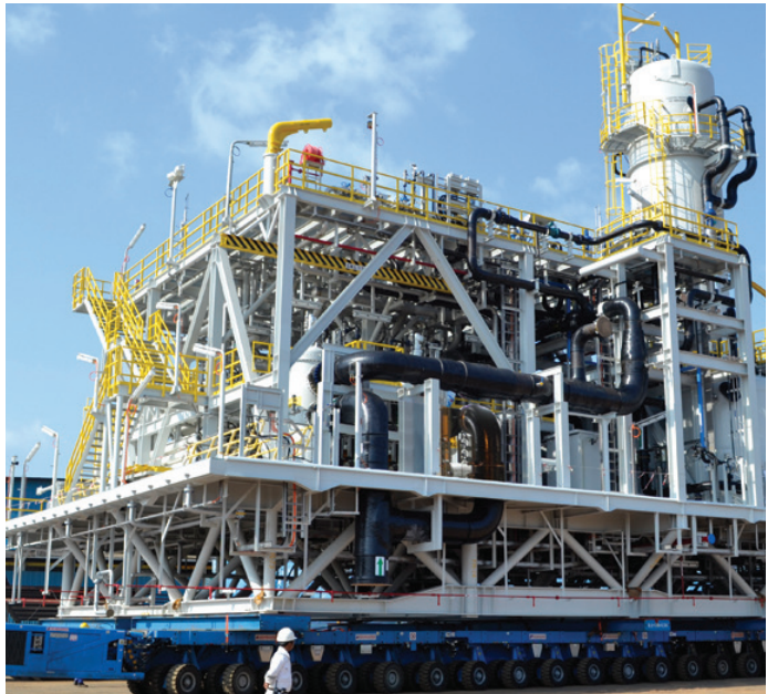
Operator/Project: Petrobras/Aker Solutions, Cernambi Sul Field Solutions Provided: Seawater Treatment Module Year Delivered: 2012
