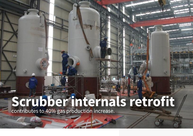
The Bellevue and Ruby Jo processing facilities were bottlenecked by poor performance of the 1st and 2nd stage scrubbers. NOV performed computational fluid dynamic simulations to demonstrate that the routing of the inlet piping and the internals design caused uneven flow distribution within the scrubber. This combined with a high gas loading resulted in liquid carryover to compressors.
