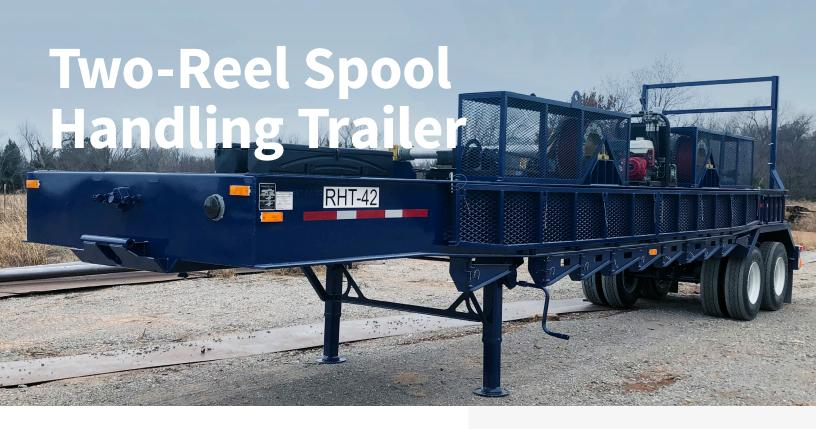
The Wilco™ two-reel spool handling trailer is designed specifically for field handling and deployment of two spools of power cable. We offer a standard package or a customized solution to meet your specific operational needs. The cable spools are Ø96-in. OD x 68-in. wide and typically weigh 20,000 lb each (40,000 lb for two cable spools). The trailer is typically used in conjunction with tensioner trailers and other equipment dedicated to deploying and assembling power cable.
