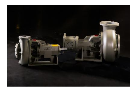
The MISSION™ Sandmaster™ line of centrifugal pumps incorporates all the abrasive-fluid handling features of the MISSION Magnum™ pump line in a more compact design, and they can be adapted for hydraulic motor drive. Compared to the Magnum, the frame and shaft have been shortened to 4 in. to reduce the pump's length.
