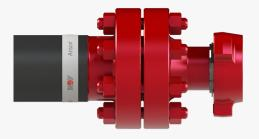
Flanged hose with Anson hammer union saver-subs Allows for quick switch outs of the low-cost saver-sub should the hammer union get damaged
