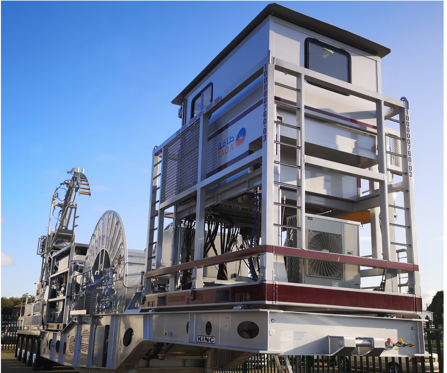
Trailer-mounted for onshore operations, this coiled tubing unit is shown with the injector upright, ready to be lifted off and craned over to the wellhead.
