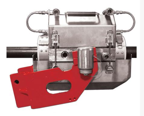
The Argus TubeSpec<sup>™</sup> coiled tubing wall thickness measuring device is a unique, patented, ultrasonic device that provides highly accurate circumferential coiled tubing wall thickness measurements as the tubing passes through the device during field operations. These measurements allow you to evaluate the coiled tubing's wall thickness, OD, and ovality along the string's length in real-time.
