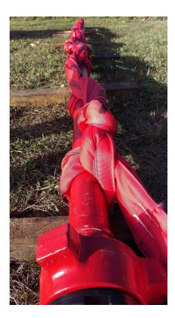
Our flowline restraint system (FRS) is a safety device designed to reduce separation between lengths of temporary pipework in the event of a pressurized pipeline rupture. The system consists of just two parts: high-strength, polyester restraints and steel shackles, and is designed for easy installation leaving a cleaner finish and look.
