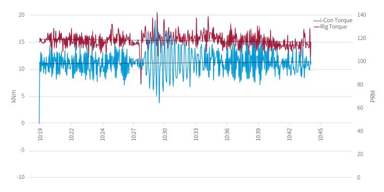
Comparing top drive torque against the logging tool data confirmed that surface values were consistently above the recorded torque from i-Con and thereby limiting the operation. After the job the rig mobilized the top drive vendor to correct the problem.
