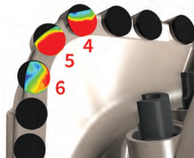
Comparison of shear stress across polycrystalline diamond compact (PDC) faces for conventional and HydroShear nozzles.
