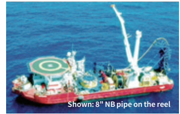
Shown: 8" NB pipe on the reel
