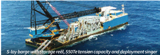
S-lay barge with storage reel, 550Te tension capacity and deployment singer
