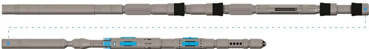
**Figure 2.** The assembly of the cup-to-cup tool.
