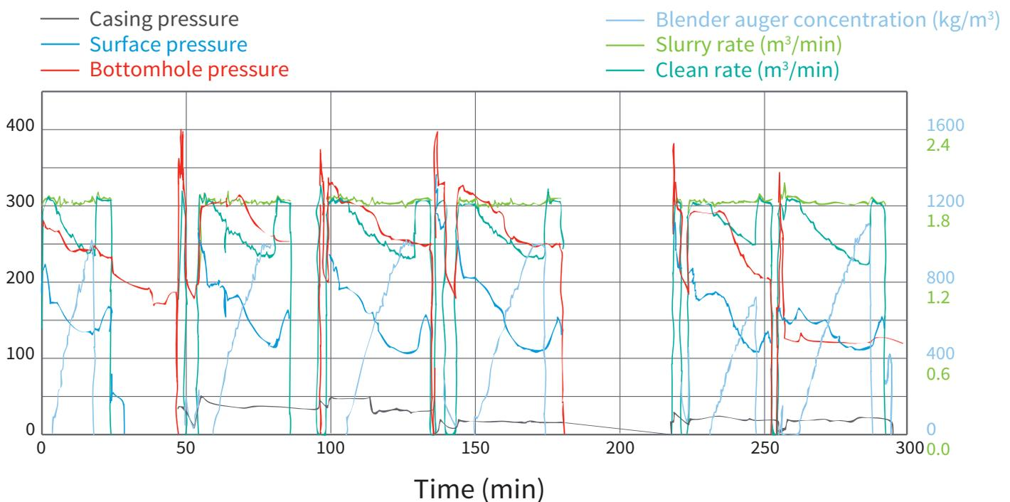
**Figure 3.** This graph provides a summary of multistage stimulation using the BPS and cup-to-cup tools, demonstrating the consistency and effectiveness of the system.
