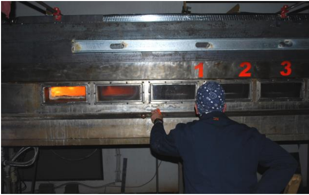
Figure 6 – Watching & Timing Flame Spread
