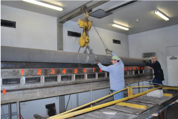
Figure 2 uPole Being Set In E84-16 Test Rig Chamber
