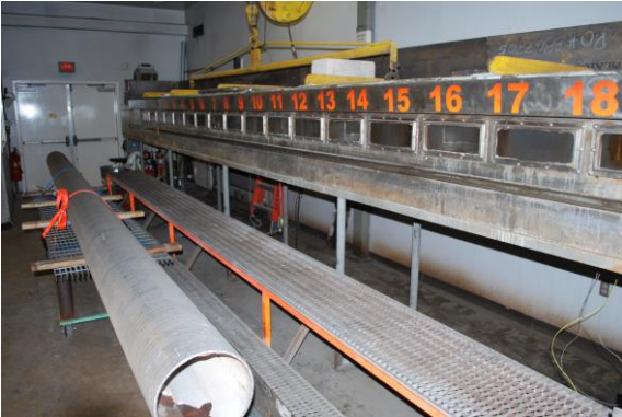
Figure 1 uPole Ready To Set in E84-16 Test Rig Chamber
