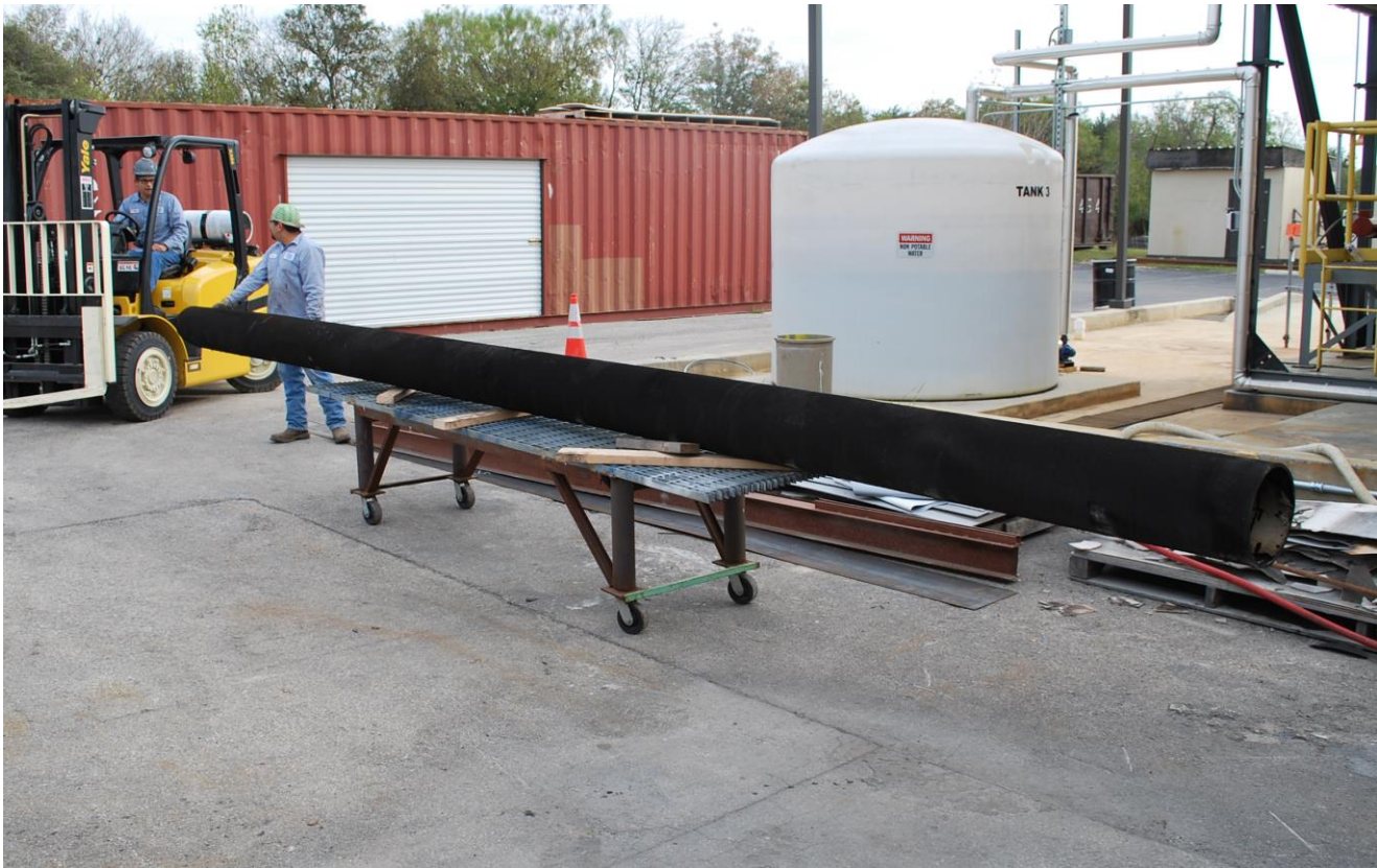
Figure 7 - Fire Tested 24 ft. Long uPole Shaft
