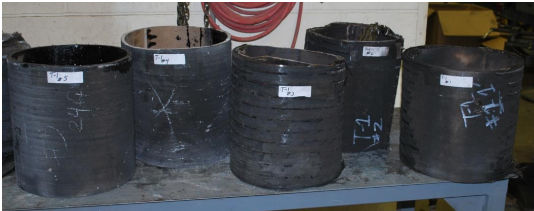
Figure 8 – Five shaft sections cut from the 10-minute E84-16 fire tested uPole shaft
