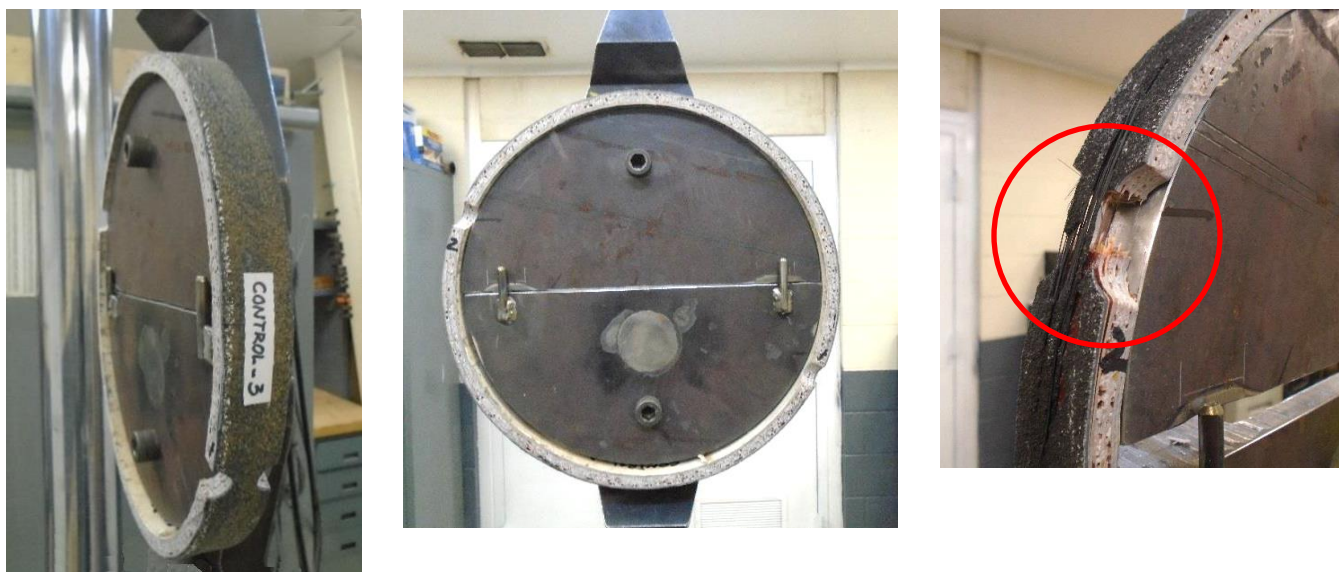
Figure 11 – Typical ASTM D2290 uPole Specimen Split Ring Hoop (90-degree) Tensile Test Setup and Mode of Break
