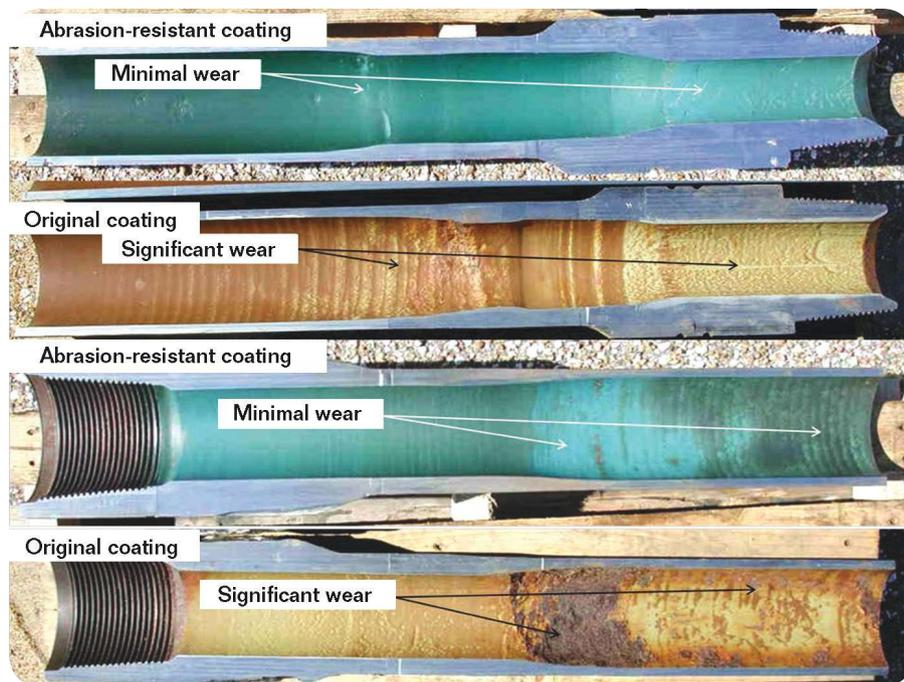
**FIGURE 1** Sections of pipe utilized in SPE 77687 comparing abrasion resistance in the same completion environment.
