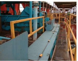
The screw conveyor is a simple way to transport drilled solids. Screw conveyors are typically used to transport drilled cuttings from the shale shaker area to a discharge port, skip or to secondary processing equipment.
