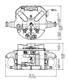
The BXS allows a safe way to run a small upset and special clearance tubulars with the new BXS elevator. This tool enables rigs to handle flush or near flush tubulars without manual intervention. The BXS provides reliable operation and is suitable for use with the FMS 275 Flush Mounted Slin
