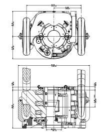
Construction of deepwater and ultra-deepwater drilling rigs created demand for equipment with a greater capacity. The BX9 has a rating of 750-1,250 sTon for 18° shoulder, 750-1,500 sTon for 90° (square) shoulder and 1,250-1,500 sTon for riser handling and 45° shouldered couplings.
