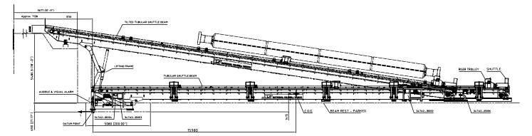
The Tubular Shuttle Machine (TS) is designed to transfer tubular between the pipe-deck and the drill-floor. Tubular can be removed from or landed onto the Tubular Beam using the elevator in combination with the front mounted Pipe Tail-in Arm. The design of the machine is basically very simple and utilizes tried and tested solutions. The design philosophy is intended to achieve minimum complexity, provide safe and reliable operation, and simplify maintenance requirements. It includes a modular
