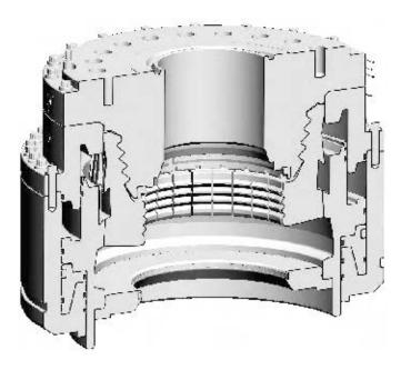
The CHX model connector is an industry leader in bending load capacity. Mechanical engagement of the unlocking piston to the finger segments, a 27% higher unlocking force to locking force, and a secondary unlocking piston ensures full release of the connector segments from the wellhead.
