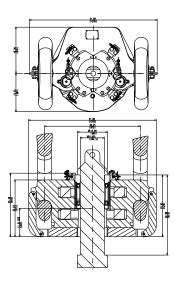
Construction of deepwater and ultra-deepwater drilling rigs created demand for equipment with a greater capacity. The SBX is a manual operated single door solid body elevator. It has a rating of 1,250 short tons for riser handling with square shouldered couplings/45° tool joints.
