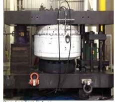
Bending Test Fixture
