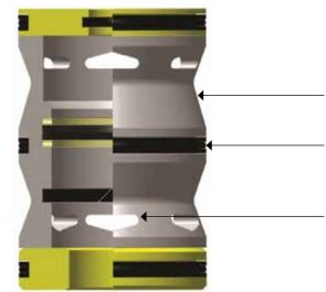
Improved cage seals (hi-gap) designed to accommodate cavity rework and larger extrusion gaps
