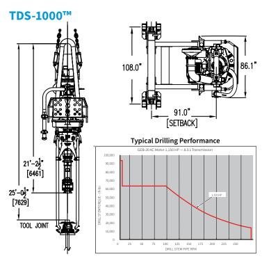
Developed for use in deep drilling applications, the TDS-1000 provides an intermittent torque output of 96,000 ft-lbs to make and break even the highest torque connections. Because of the broad speed and torque range provided by the AC motor, this performance is obtained using a single-speed gear box. The TDS-1000 Top Drive is driven by a Variable Frequency Drive (VFD) control system for a greater range of torque and speed performance.
