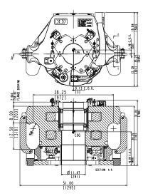
Construction of deepwater and ultra-deepwater drilling rigs created demand for equipment with a greater capacity. The BX7 has a rating of 1,000 short tons for drill pipe and landing strings, and 1,250 short tons for riser handling and square shouldered couplings.
