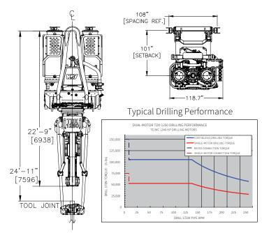
The TDX 1250 combining the best of the NOV leading top drive brands with new technology, the TDX includes high reliability systems like water cooled, flameproof motors with quick decouple drive connections, easily removable main shaft with a huge NC84 connection, and a massive 1,236 ton API main bearing in a wet-sump gearbox. These all add up to improved reliability and increased uptime. The TDX also brings many revolutionary innovations such as the "FlexFit" link
