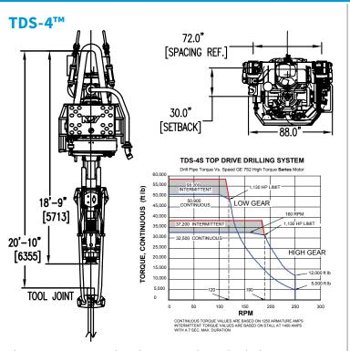
The TDS-4S is our prime large bore DC top drive. It has built its reputation by performing will in the heavy drilling environments found offshore. This 750 ton top drive has been in service and operation since 1988 and over 350 units have been in service since that time. Although considered a mature product, its high demand in the top drive market today is a tribute to its robust and reliable reputation built on years of drilling experience.
