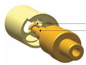
Key/keyhole design eliminates retainer nut
