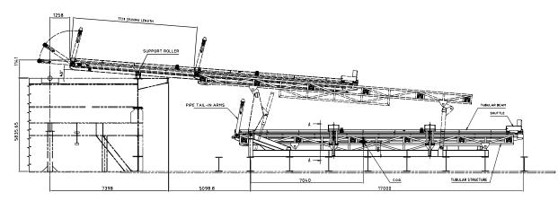
The Tubular Shuttle Machine (TS) is designed to transfer tubulars between the pipe-deck and the drill-floor. Tubulars can be removed from or landed onto the tubular beam using the elevator in combination with the front mounted Pipe Tail-in Arm. The design of the machine is basically very simple and utilizes tried and tested solutions. The design philosophy is intended to achieve minimum complexity, provide safe and reliable operation, and simplify maintenance requirements. It includes a modular
