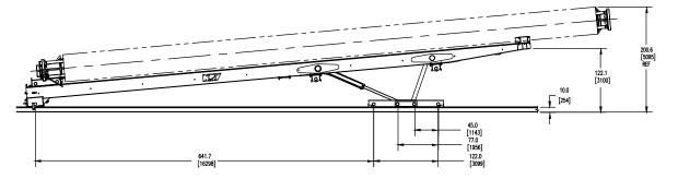
The Riser Handling System (RHS) uses a hydraulically powered trolley-on-atrolley to accomplish two tasks. (1) Transporting horizontal riser joints from the riser deck to the well center. (2) Safely tailing the riser section while it is hoisted by the drawworks from a horizontal to vertical position. The system can accommodate various requirements of riser length, diameter, and riser spider/gimbal height.
