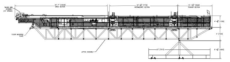
The Pipe Transfer Conveyor (PTC-LD) is a light duty conveyor with an attached Tailing Arm Assembly. The PTC transports drilling tubulars between their storage location on the main pipe deck and well-center without manual intervention from the rig crew. It can be remotely operated from the rigs main control cabin through integrated controls or operated locally from a local control station. The PTC has two main sections: Conveyor & Tailing Arm Assembly.
