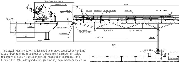
tubular both running in- and out of hole and to give a maximum safety to personnel. The CWM gives an almost "hands-free" operation of the tubular. The CWM is designed for rough handling, easy maintenance and a long trouble free operation time. The CWM is built as one unit to minimize installation costs on the rig.
