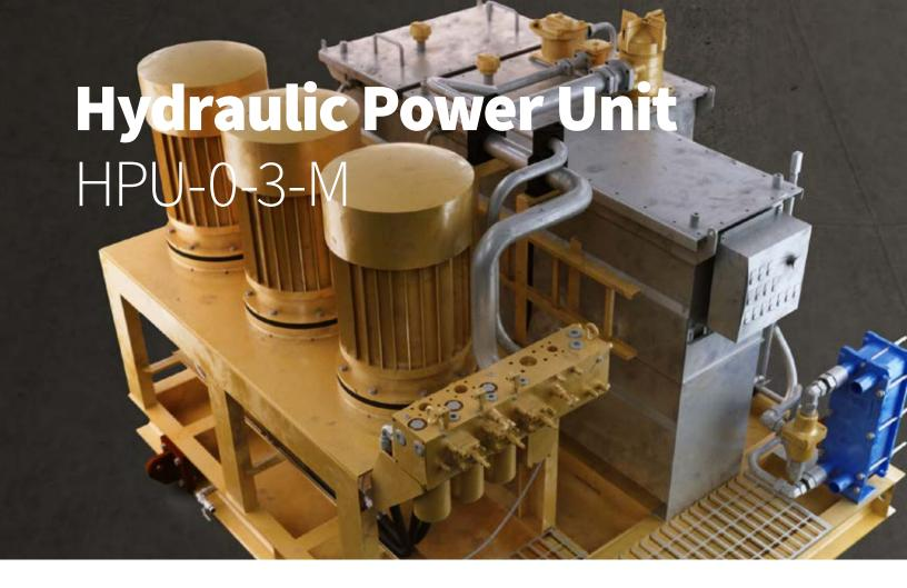
The Hydraulic Power Unit is a skid-mounted freestanding unit designed to feed high pressure hydraulic oil with acceptable cleanness to the vessel ring line system and applicable drilling equipment. The ring line system is an open loop hydraulic system. The HPU may be operated locally at the unit.
