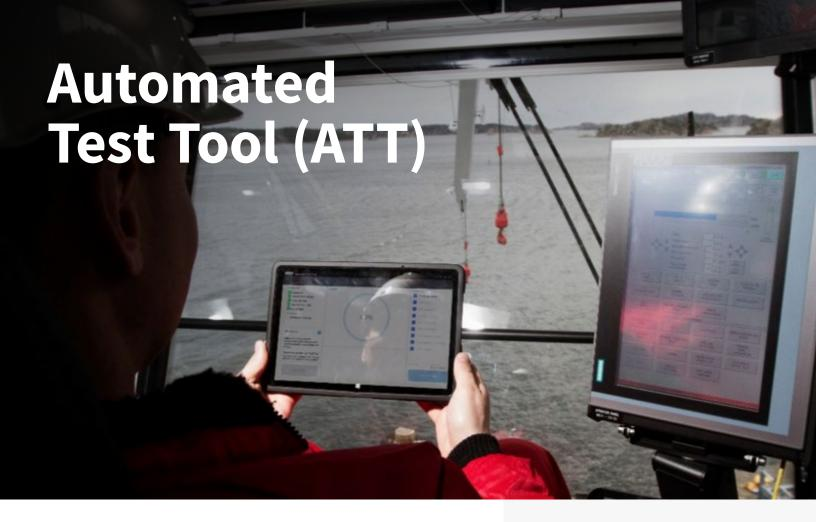
The Automated Test Tool (ATT) for cranes comprises a suite of customizable software applications that enable you to verify and document critical crane functions. By detecting and identifying potential failures before they happen, the ATT reduces operational downtime while enabling optimum system performance. That's less time and money spent on regular inspections and more cost savings overall.
