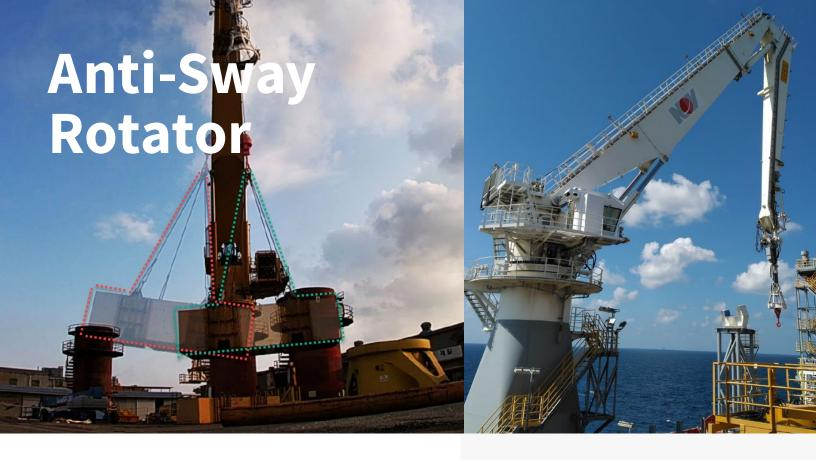
Load control during a lift operation requires considerable crew intervention to reduce the load sway and rotate and place the load in the desired location. The Anti-Sway Rotator (ASR) enables a more efficient and safer lift operation, reducing overall costs.
