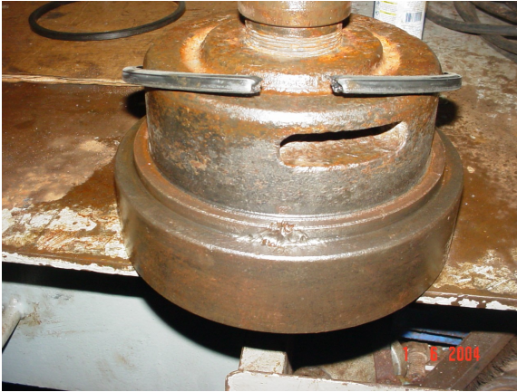
Gasket Installed on Worn Valve Cap and Not Greased Prior to Operation
