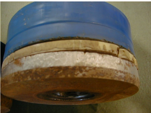
Blue Lightning Heat Damage
