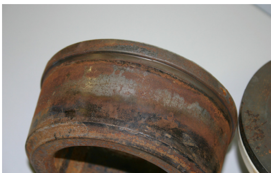
Poor Taper Contact API Taper Pump
