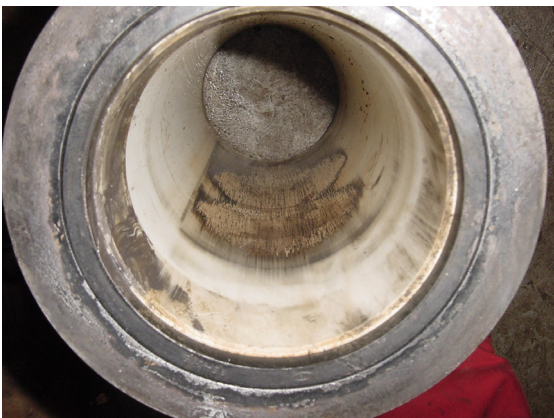
Photographs of scoring in liner bore disrupting ceramic surface.
