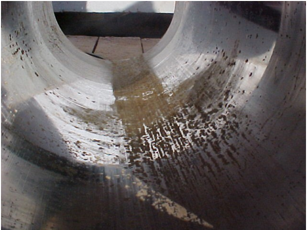
Liner operated in acidic or caustic fluid.
