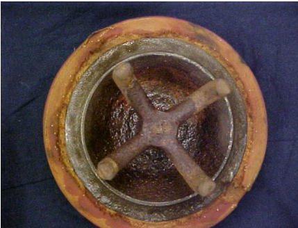
Roughneck Extrusion Damage
