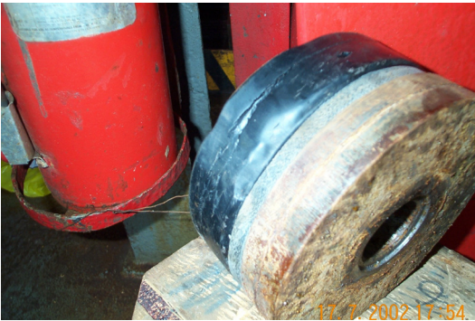
Heat Damaged Piston
