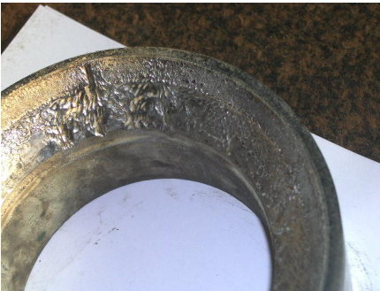
Roughneck Seat Corrosion
