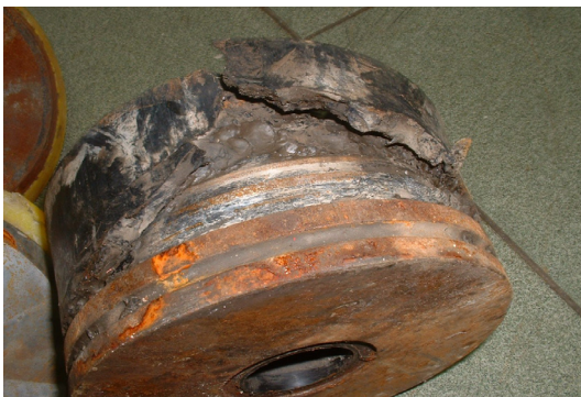
Flex Lip in a Worn Out Liner
