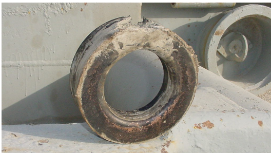
Photographs of a Piston Rubber Operated on a Worn Out Piston Body
