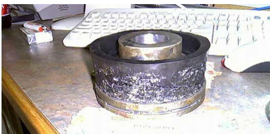
Flex Lip Heat Damage
