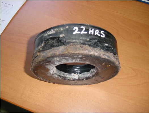
Rubber Extrusion Damage
