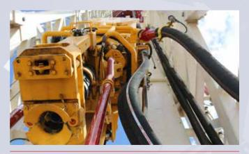
**Figure 2.** The TDS-11SAE is powered by two new 600 hp induction motors, increasing power for use in ERD wells. Image provided by NOV.
