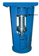
Less than 0.5" gap resulting from drop into mounting flange catcher bracket
