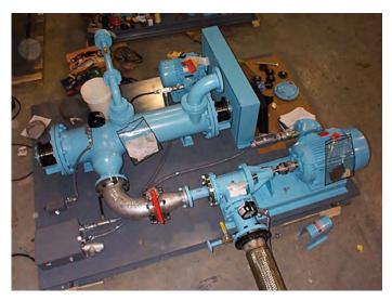
Greerco Pipeline mixers can easily be placed into an existing system to increase efficiency
