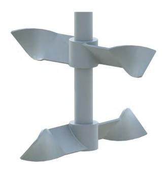
The JT-2 impeller is used for superior blending in transitional flow. High viscosity and non-Newtonian fluids make blending much more challenging. This impeller is used after conventional turbines have lost efficiency due to viscous effects and before the need for close clearance impellers.
