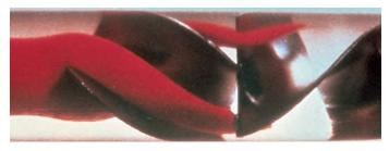
The Kenics heat exchanger directs the flow of material radially toward the pipe walls and back to the element for the most efficient thermal transfer
