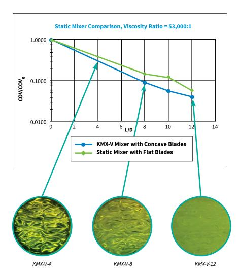
Laser induced fluorescence (LIF) images showing cross-sectional uniformity
