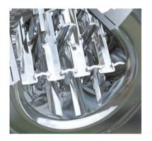
Low viscosity additives are driven along the trough of each blade and abruptly sheared by strong cross-stream velocity gradients as they pass around the upstream surface
