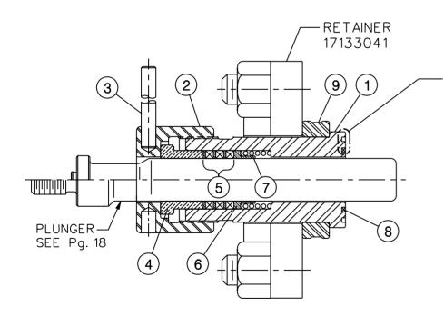
250T- 5H  $2\frac{1}{8}$ ", 2" &  $1\frac{7}{8}$ " PLUNGER KIT WITH CLAMPED OR THREADED PLUNGER
