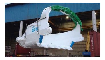
We also manufacture truck bodies, water tanks, and large dragline and dipper buckets for our mining customers. All welding qualifications and compliance are according to AWS D1.1 and/ or AS1554-1 & 4. We use only the highest quality wear-resistant, high-tensile quenched and tempered plates to fabricate all truck bodies at our facility in Batam.
