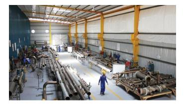
We can prefabricate piping spools for onshore and subsea applications from a variety of materials. We can also fabricate associated supports and structures, such as walkways and access platforms, and deliver clad pipe and fittings to support corrosive environments.
