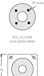
1C2 slotted base plate prestressed to pole
