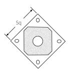
1C5 diamond pattern slotted base plate prestressed to pole
