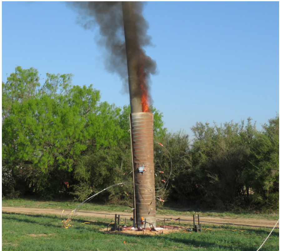
Enhanced Ameron uPole fire test, 2-minute exposure
