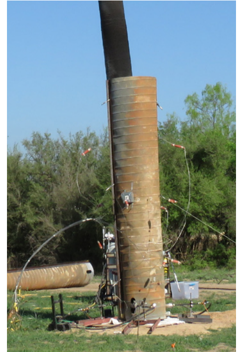
Fire test set up with shroud, instrumentation, and propane torches
