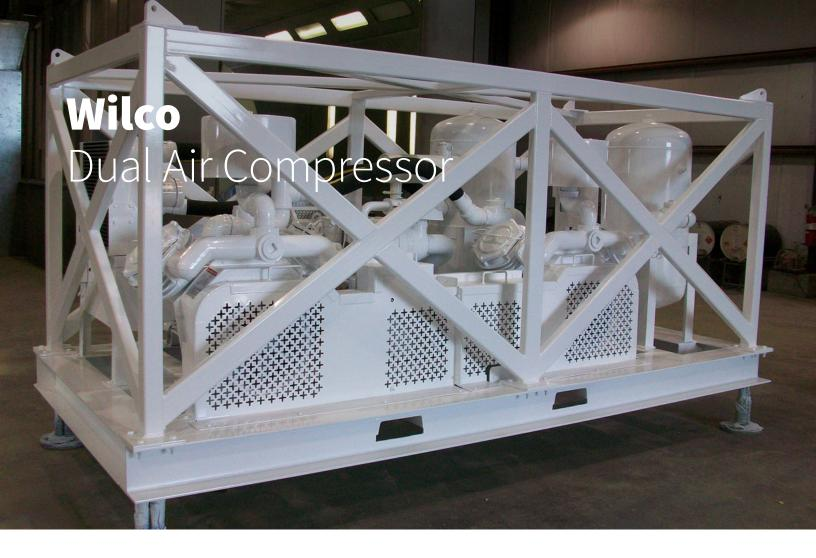
The Wilco<sup>™</sup> dual air compressor is skid-mounted with dual cylinder pumps and produce 410 ft<sup>3</sup>/min (680 m<sup>3</sup>/hr) at 1,072 RPM.
